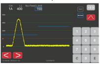
To find the no-feed limit, run the roller with parts and hold them back in the rail to simulate a no-feed. With parts, the average is 498; holding them can gives an average of 4. Set the no-feed limit to 8; if it drops below 8, the die area is empty.
