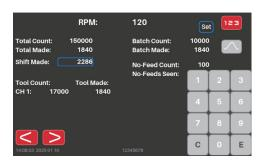
Press the **123 Button** to bring up the count view/adjustment display.
